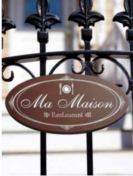
V-Carving mode produces sharp angles for three-dimensional lettering with a hand-crafted look.
