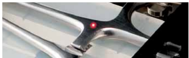
▲ Confirm the correct marking location with the built-in laser pointer
